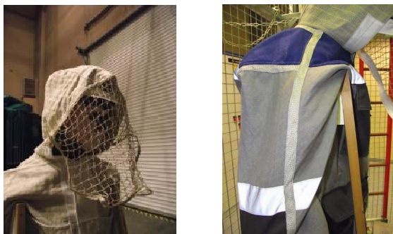
Figure 9: additional face mesh and metal threads on a conductive clothing
